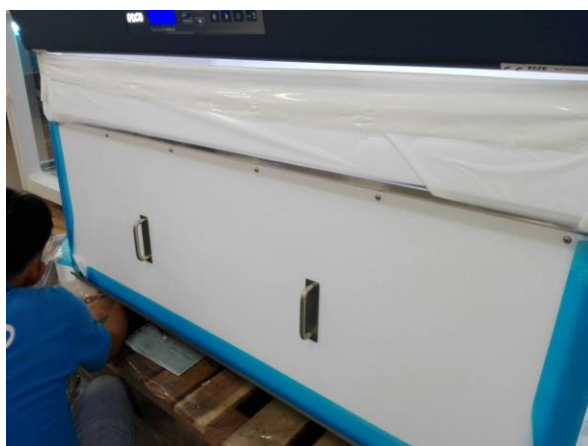
Figure 1. A front cover blocking the UV Light for protection of investigators.
