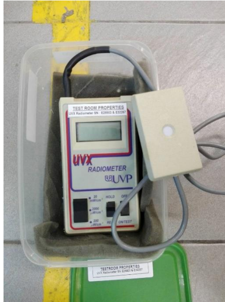
Figure 3. Radiometer used for UV measurement.
